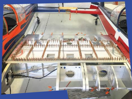
The custom center section was designed and fabricated entirely from scratch.
